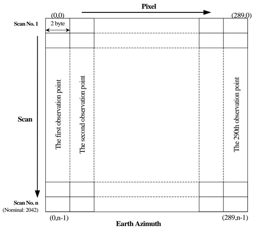
Figure 1.2-9 The Structure of Earth Incidence, Earth Azimuth
