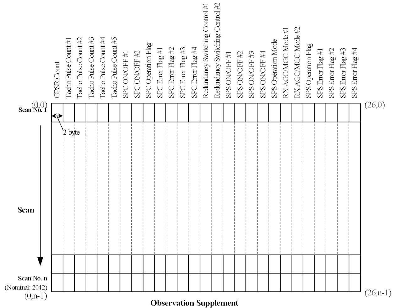
Figure 1.2-11 The Structure of Observation Supplement
