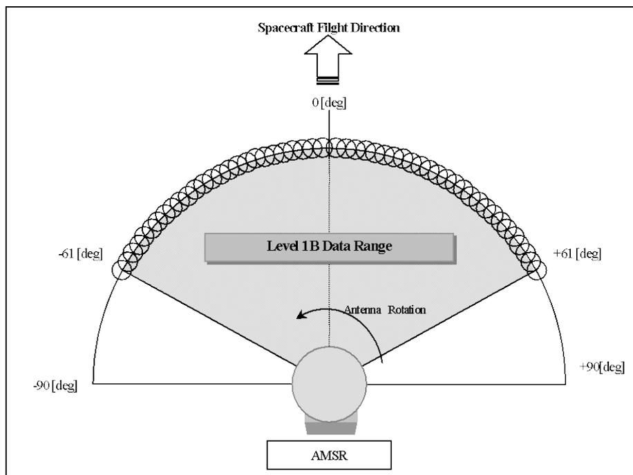
Figure 1-1 Range of one scan for AMSR (Level 1B)
