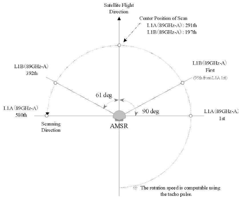
Figure 3.1-2 Geometry of the observation points of a scan
