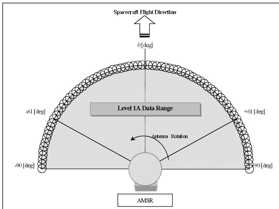
Figure 1-1 The range of one scan for AMSR (Level 1A)
