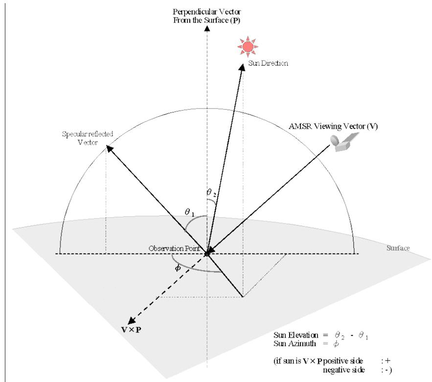
Figure 2.3-1 The definition of Sun Elevation, Azimuth
