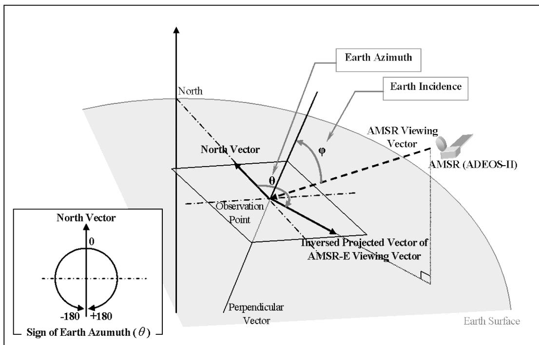
Figure 2.3-2 The definition of Earth Azimuth, Incidence
