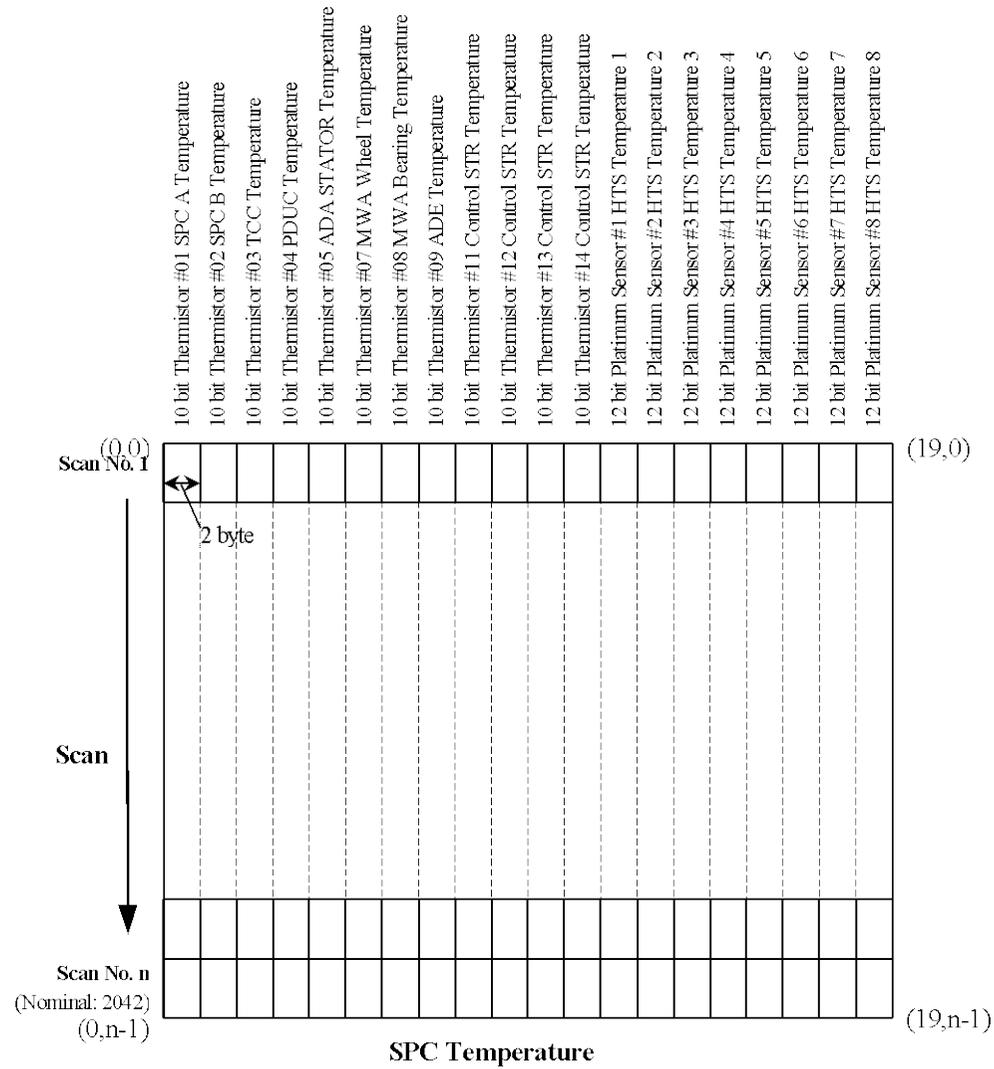
Figure 1.2-12 The Structure of SPC Temperature Count
