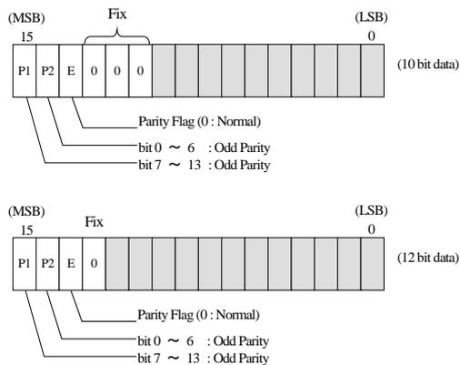
Figure 2.3-4 The Data Structure of SPS Temperature Count
