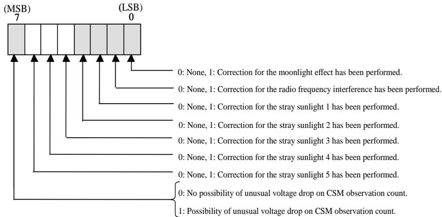
Figure 2.3-6 The Format of The Interpolation Flag
