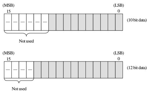
Figure 2.3-3 The Data Structure of SPC Temperature Count
