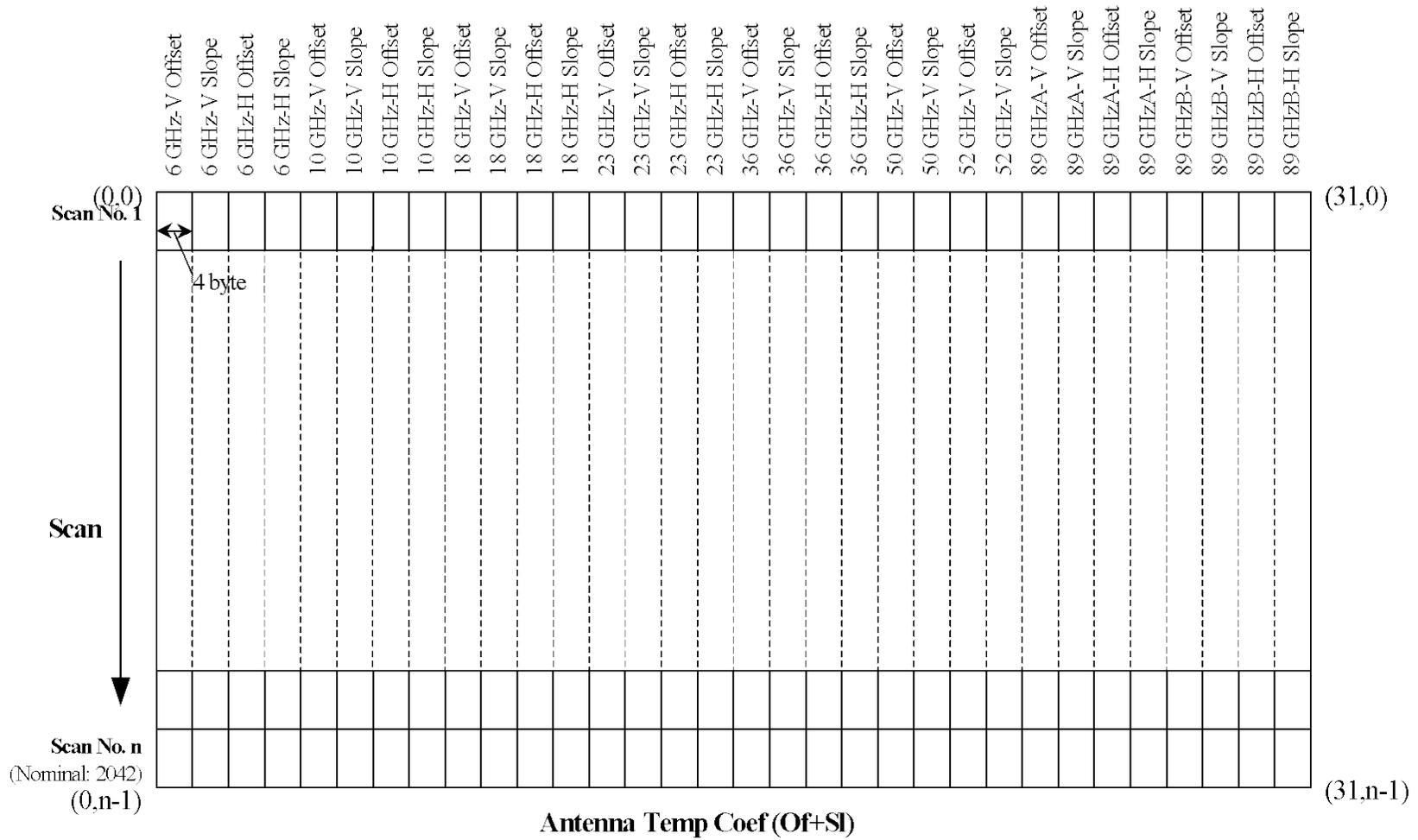
Figure 1.2-5 The Structure of Antenna Temp Coef
