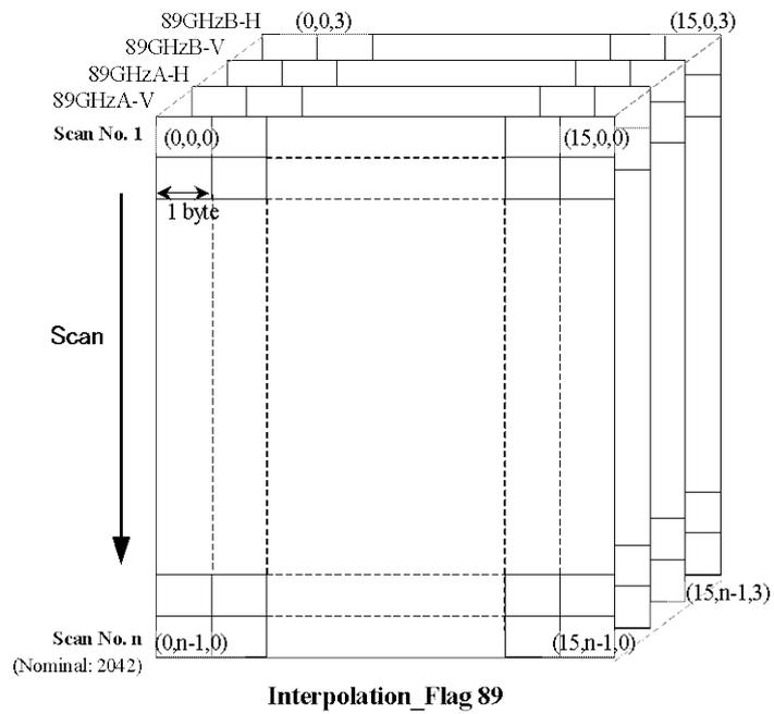
Figure 1.2-15 The Structure of Interpolation Flag
