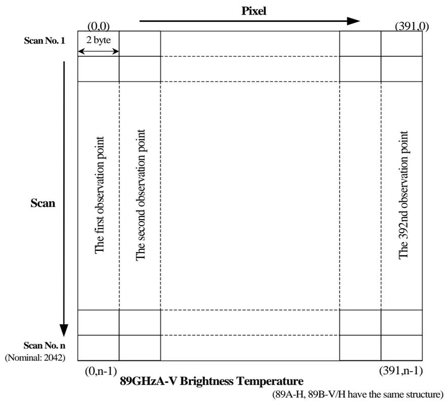
Figure 1.2-2 Structure of Brightness Temperature
