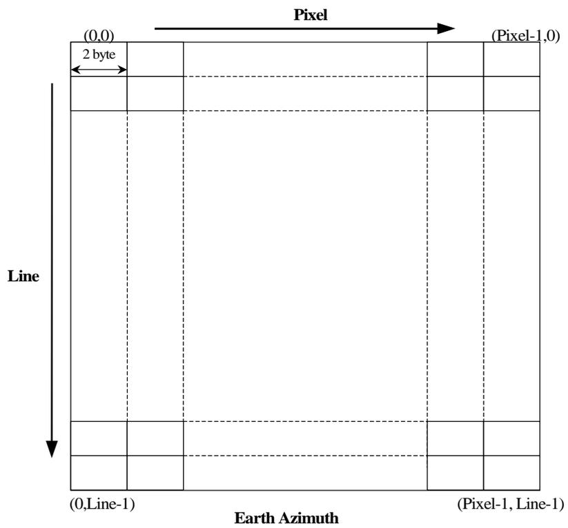
Figure 1.2-4 Structure of Earth Incidence and Earth Azimuth
