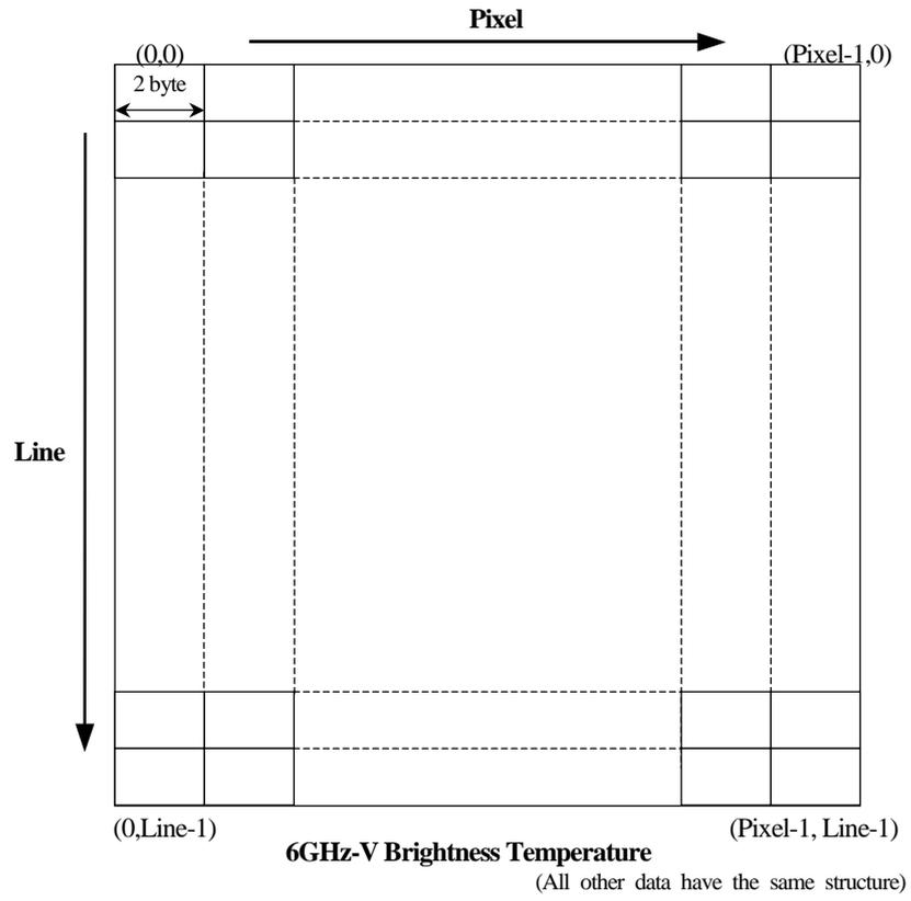
Figure 1.2-2 Structure of the Mapped Brightness Temperature (Image Data)
