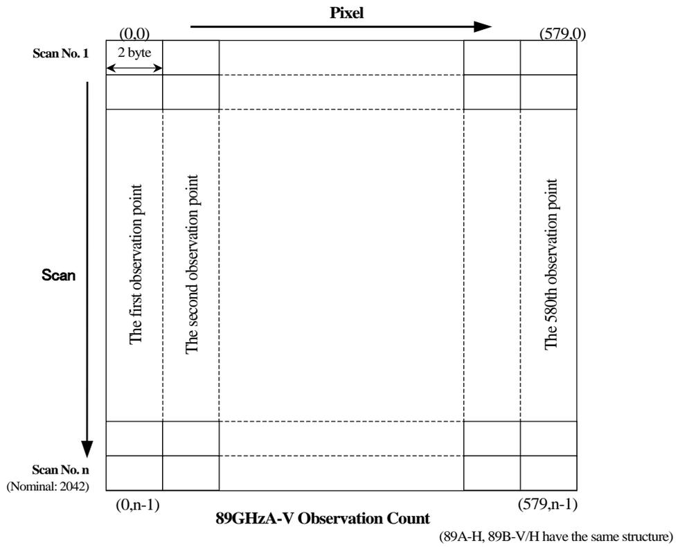
Figure 1.2-2 The Structure of Observation Count
