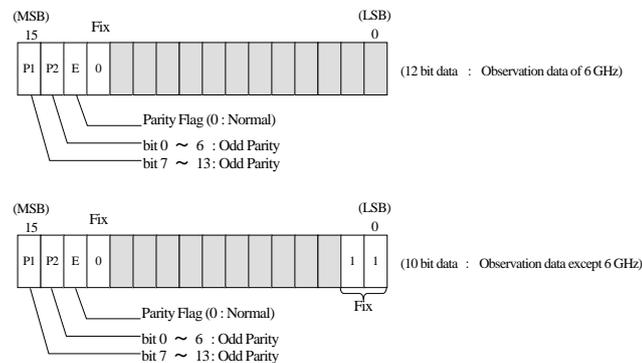
Figure 2.1-2 SPS Temperature Count data
