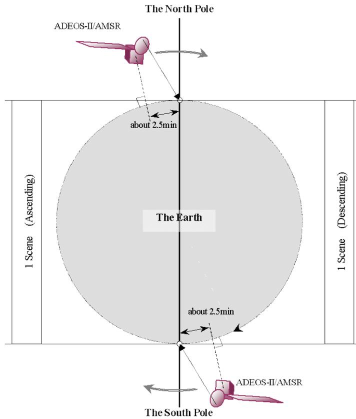
Figure 3.1-1 Geometry of a scene and the flight direction of ADEOS-II
