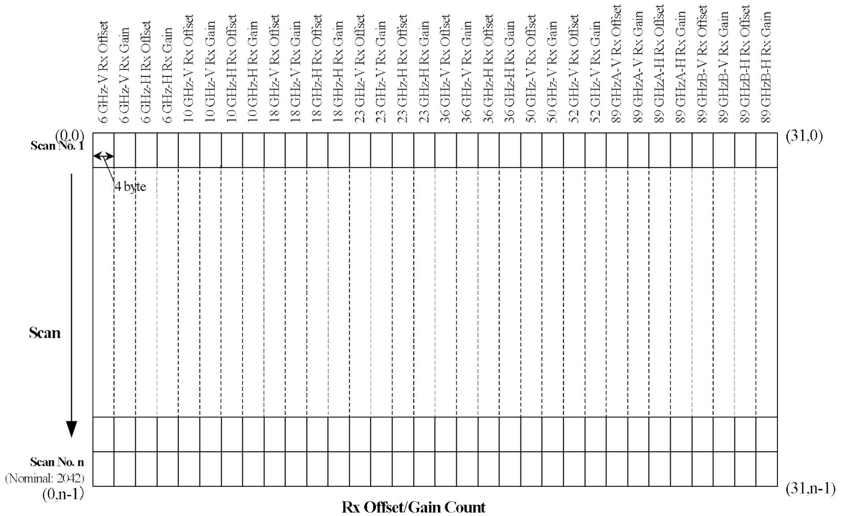
Figure 1.2-6 The Structure of Rx Offset/Gain Count
