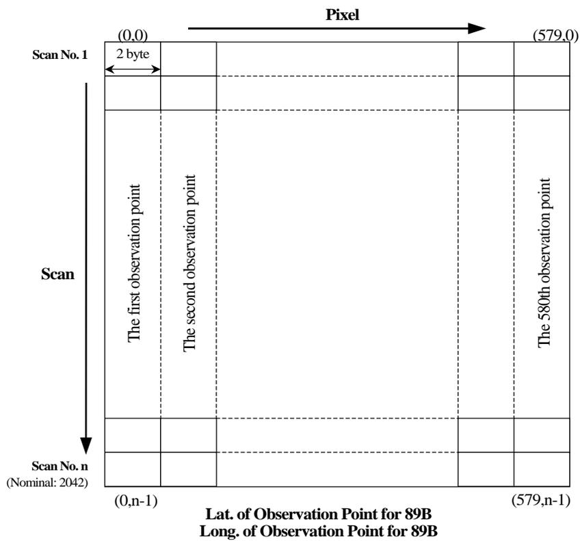
Figure 1.2-7 The Structure of Lat of Observation Point, Long of Observation Point
