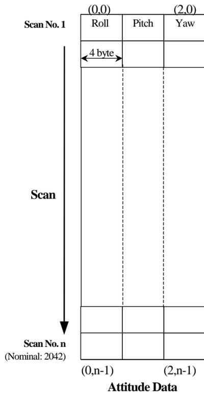
Figure 1.2-4 The Structure of Navigation Data, Attitude Data
