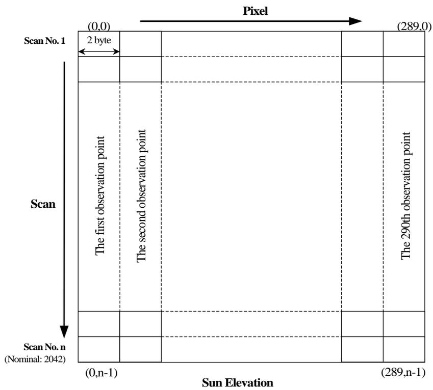
Figure 1.2-8 The Structure of Sun Azimuth, Sun Elevation
