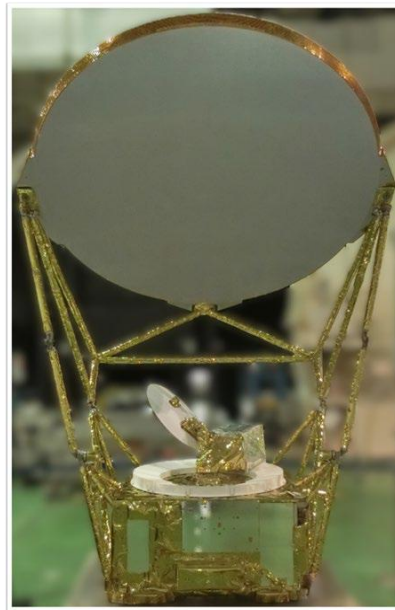
Figure 2-3 Exterior views of AMSR3
